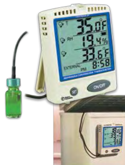
Thin cable makes it easy for refrigerator door to close and seal
