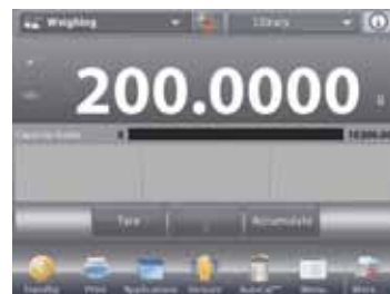
High resolution, 5.7" color TFT display
