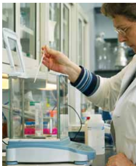
Removable front, side and back glass panels
