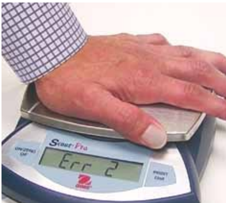
Mechanical and software overload protection
