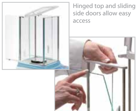
Removable front, side and back glass panels
