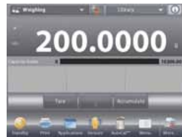
High resolution, 5.7" color TFT display
